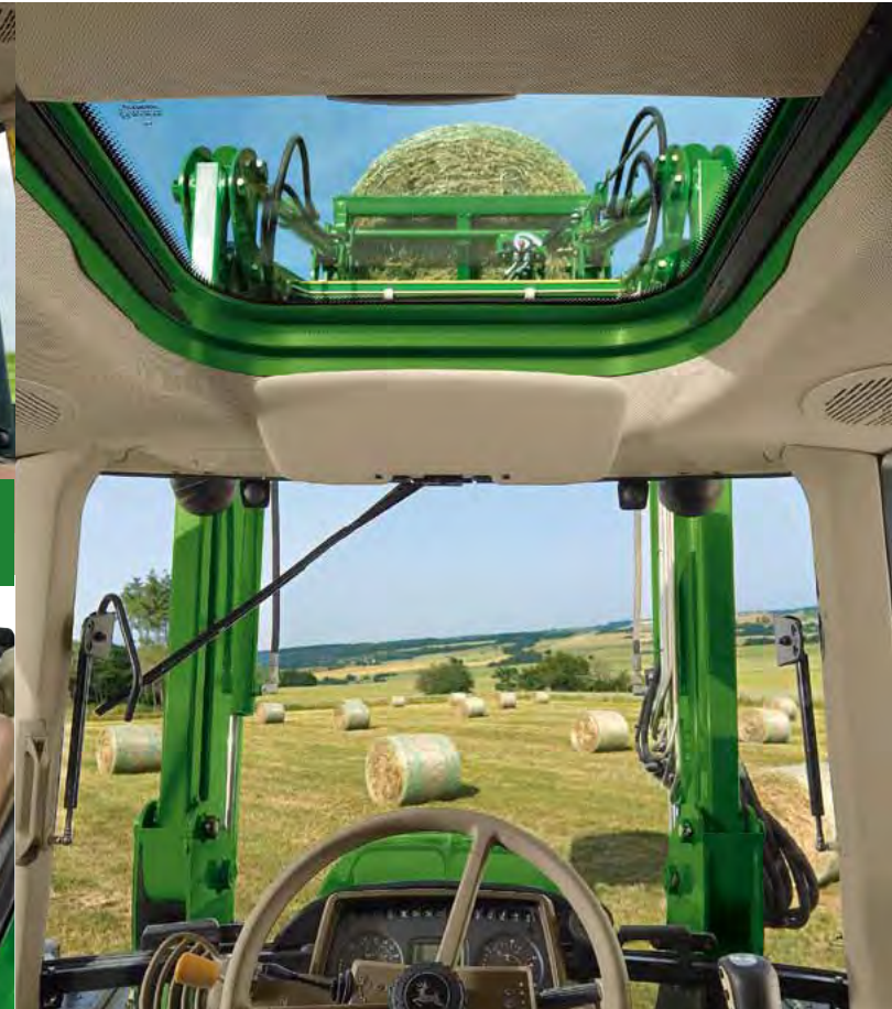
Optional tiltable front windshield can be adjusted to improve cab air flow.
