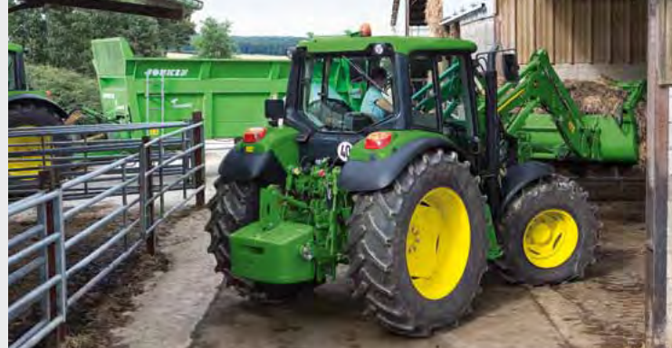
PowrReverser™ 16/16 has 16 forward and 16 reverse speeds, plus a left-hand reverser (on selected versions) for clutchless direction changes that speed up loader work.
