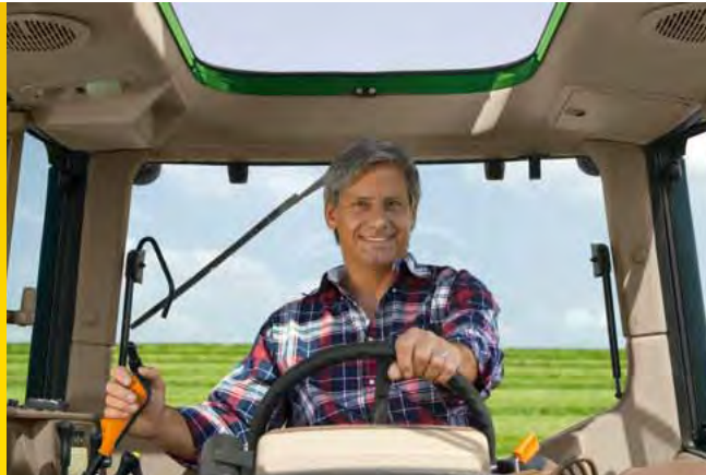
Optional roof hatch with glass makes it easy to see loads that are normally out of sight when working in tight, low buildings.
