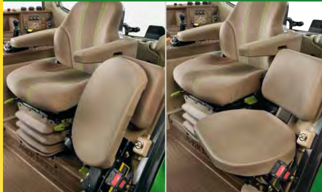
Optional instructional seat can be folded out of the way when not in use.
